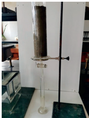
Figure 3. Laboratory experiment for water permeability
