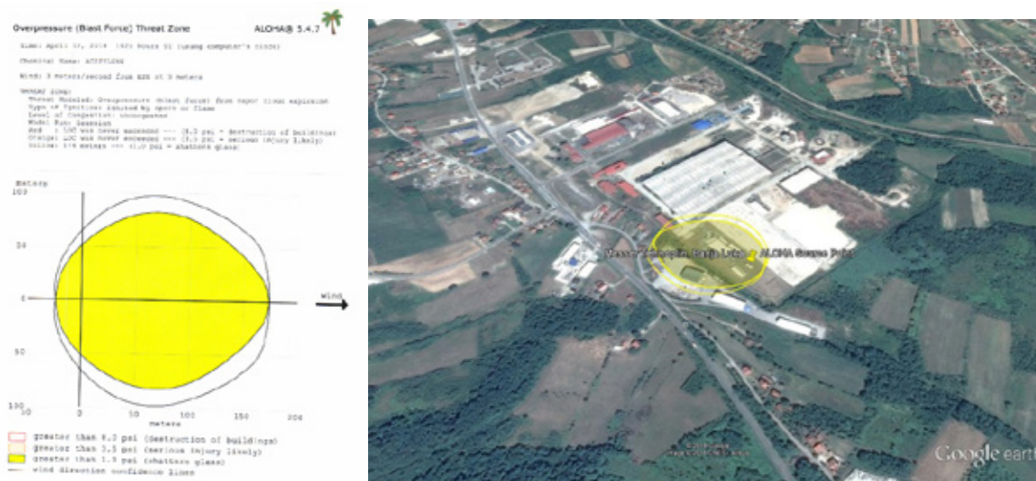
Figure 5. Over-pressure due to Acetylene Explosion and Examples of scenario Steam Cloud effects for acetylene
