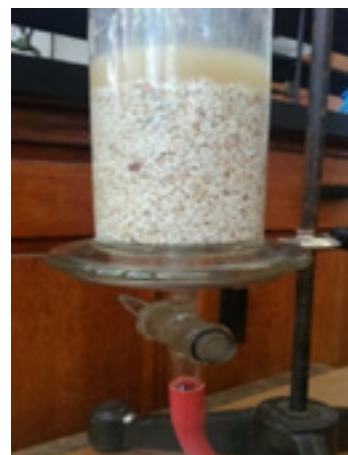
Figure 5. Filtration layers of WOT
