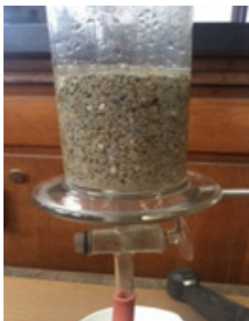
Figure 4. Filtration layers of DE
