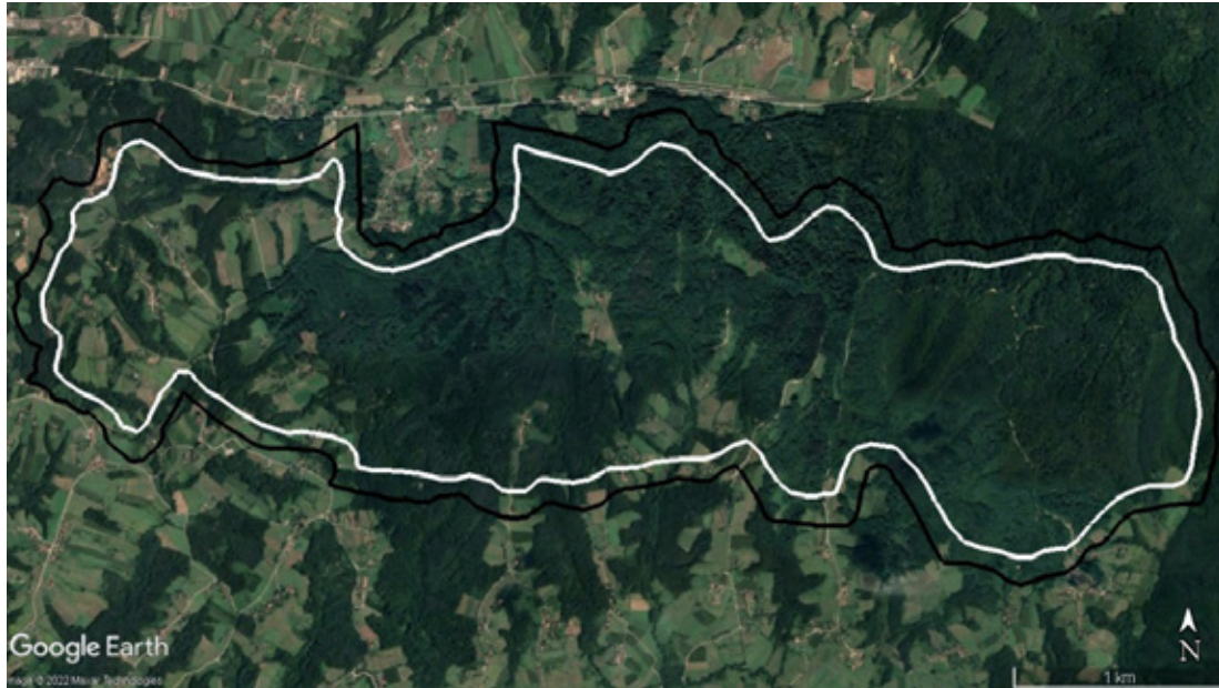
Figure 1. The black solid line represents the exploitation front. The area between the black and white lines is the noise protection zone created of the Ostružnja surface mine
