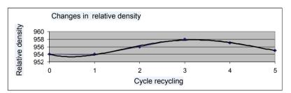
PICTURE 2. SHOWING THE CHANGES OF CHARACTERISTICS OF POLYETHYLENE
